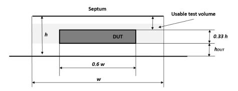
When rotating the DUT into any of the three main orthogonal positions, the geometrical center of the electronic section of the device shall remain in the same position.
