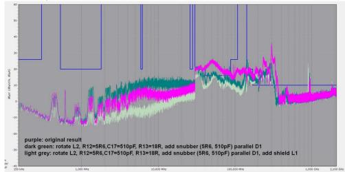
Example: using a TEM-cell and EMCview software to track the effects of hardware modifications over a wide frequency range
