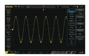
Built-in dual-channel 25 MHz source (DS1XX4Z-S Plus)
