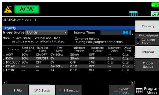
**3** Use the numeric keypad or the rotary knob to enter the time.
