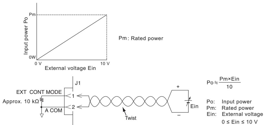
To avoid noise interference, use a highly stable, low-noise external voltage source and twisted signal wires.
