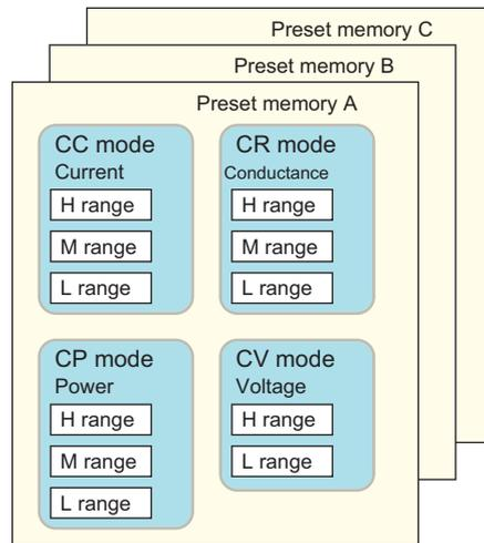
For example, when you save to preset memory A in CC+CV mode (current: M range, voltage: L range):
