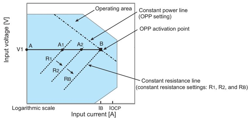
If the overcurrent protection (OCP) setting  $IOCP$  is greater than the current value  $IB$  at point B, when the PLZ-4WL resistance is decreased ( $R_1 \rightarrow R_2 \rightarrow R_B$ ) so that the input current (load current) increases, with the voltage of the constant-voltage power supply at  $V_1$ , the operating point moves along segment AB ( $A_1 \rightarrow A_2 \rightarrow B$ ). When point B is reached, overpower protection (OPP) is activated.
