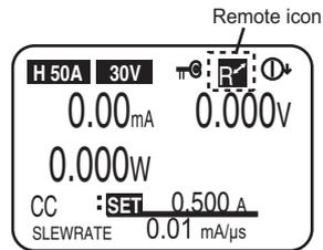
When the PLZ-4WL is in remote mode, the remote icon appears on the display. To use the front panel to switch the PLZ-4WL back to local mode, press LOCAL.
