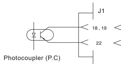
Use pins 18 (RANGE STATUS 1) and 19 (RANGE STATUS 0) of the J1 connector (pin 22 is common).
