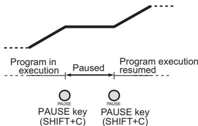
Example: Pause by executing PAUSE in a program, and resume using trigger input (TRIG IN).
