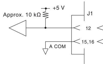
Apply an external signal to pins 12 and 15 or 12 and 16 of the J1 connector.
