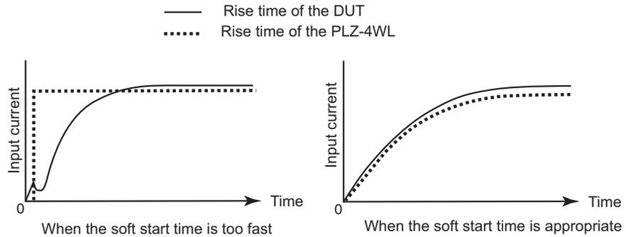
If the current rise time that is determined by the slew rate and the current setting is longer than the soft start time, the actual rise time will be longer than the soft start time. If you want to raise the current according to the soft start time, increase the slew rate.
