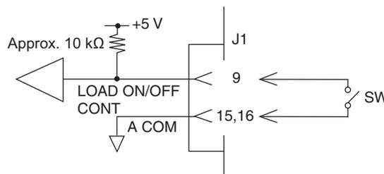
The input pin is pulled up to the internal circuit's +5 V level by a resistor that is approximately 10 kΩ. The maximum allowable voltage is 5 V. The logic threshold levels are CMOS.
