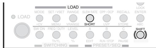
If you press SHORT (SHIFT+SLEW RATE) while the short function is off, the short icon is displayed, and the short function turns on. In constant current mode (CC mode), the fundamental setting is set to the maximum current value; in constant resistance mode (CR mode), the fundamental setting is set to the minimum resistance value.
