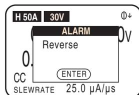
The protection functions are activated when a reverse voltage of approximately 0.4 V or greater is applied. If this happens, turn off the DUT immediately.
