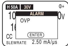
The maximum voltage that can be applied to the load input terminals is 30 Vdc. You cannot use voltages that exceed 30 Vdc. When excessive voltage is applied, the protection functions are activated. Lower the voltage of the DUT immediately.
