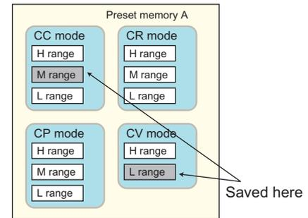
In CC+CV mode, memory entries for CC mode and CV mode are used.
