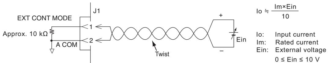
To avoid noise interference, use a highly stable, low-noise external voltage source and twisted signal wires.
