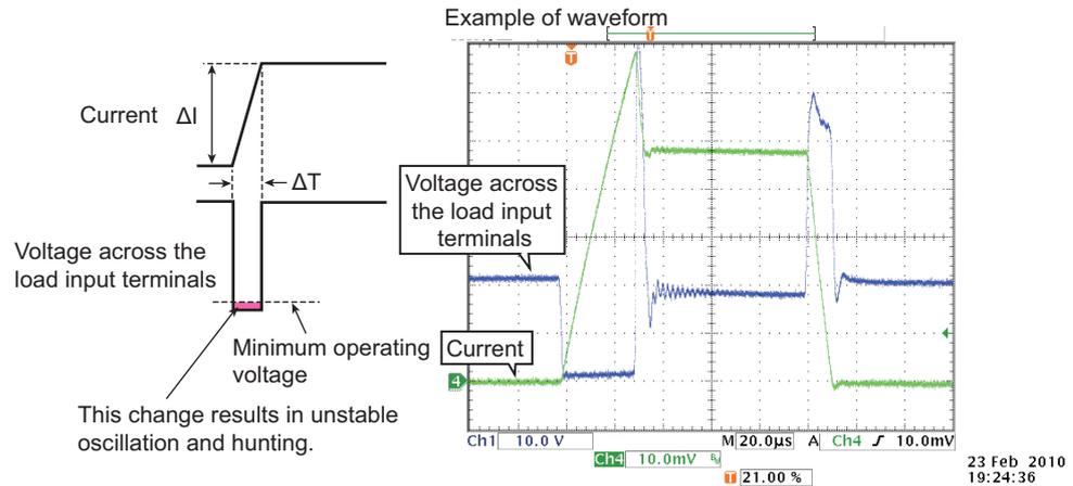
To make sure that the voltage resulting from inductance remains within the range of the electronic load's minimum operating voltage and maximum input voltage, make the wiring as short as possible and twist the wiring, or reduce the slew rate. If it is not necessary to operate at a high response speed, reduce the slew rate in CC mode, or reduce the response speed in CR mode.
