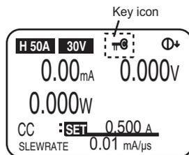
If you press LOCK (SHIFT+LOCAL) when the key icon is not displayed, the keys are locked, and the key icon appears.
