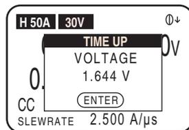
In voltage measurement, the voltage immediately before the load turns off is measured. You can configure the PLZ-4WL to turn the load off after a specified amount of time has elapsed. After the load turns off, a popup window appears indicating the input voltage immediately before the load was turned off.
