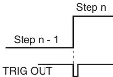
Example: Set trigger output at step number n (TRIG ON).
