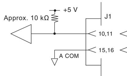
Use pins 10 (RANGE CONT 1) and 11 (RANGE CONT 0) of the J1 connector (use pin 15 or 16 as the common).
