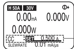
Constant current (CC) mode is selected in this screen, so you can enter the current, which is the fundamental setting.
