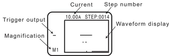
Each time you press ▼, the cursor moves between items in this order: step number, current, trigger output setting, and then magnification.
