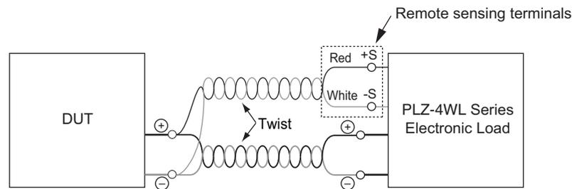
The table below indicates sizes of the wires that you can use to connect to the sensing terminals. Strip approximately 10 mm of coating from the end of the wiring.
