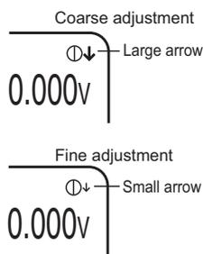
Use the rotary knob to set values such as the current and resistance. Turning the rotary knob clockwise increases a value and turning it counterclockwise decreases the value.
