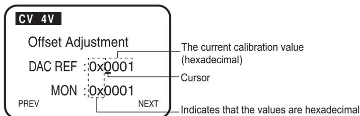
**4 Press ◀ or ▶ to set the cursor position of DAC REF, and then turn the rotary knob so that the input voltage is within  $\pm 0.05$  % of the value corresponding to 10 % of the full scale value (see the table of CV mode settings).**
