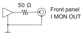
The common is connected to the chassis electric potential. It is isolated from A COM. For current ranges H and L, 1 V corresponds to the full scale current; for current range M, 0.1 V corresponds to the full scale current. The output impedance is approximately 50  $\Omega$ .
