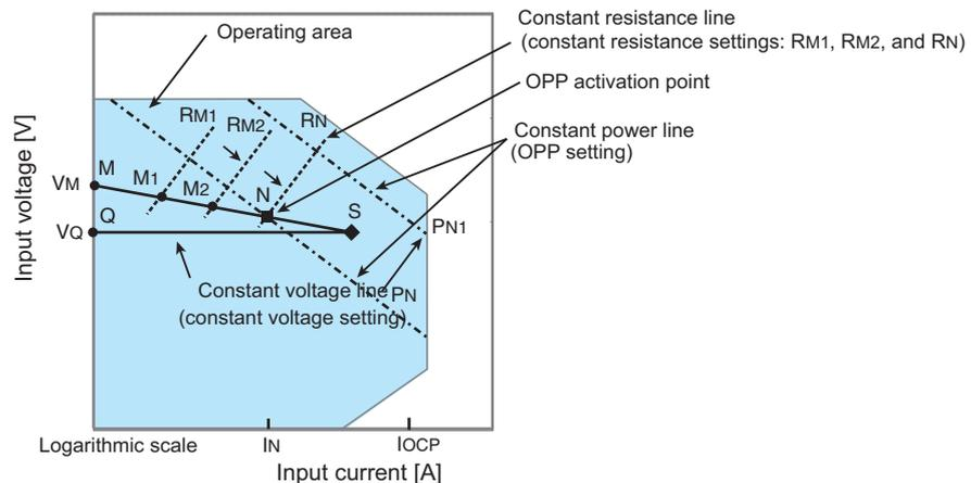
When the overcurrent protection (OCP) setting  $I_{OCP}$  is greater than current  $I_N$  at point N, the voltage of the battery is  $V_M$ . In constant resistance (CR) mode, if the resistance is reduced ( $R_{M1} \rightarrow R_{M2} \rightarrow R_N$ ) so that the input current (load current) increases, the operating point moves along segment MN ( $M_1 \rightarrow M_2 \rightarrow N$ ).
