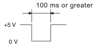
Input a signal with a pulse width of 100 ms or greater.
