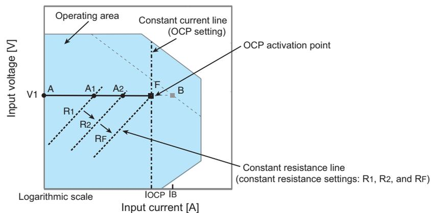
If the overcurrent protection (OCP) setting IOCP is less than the current value IB at point B, when the PLZ-4WL resistance is decreased ( $R_1 \rightarrow R_2 \rightarrow R_F$ ) so that the input current (load current) increases, with the voltage of the constant-voltage power supply at V1, the operating point moves along segment AF ( $A_1 \rightarrow A_2 \rightarrow F$ ). When point F is reached, overcurrent protection (OCP) is activated.
